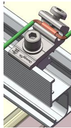
Fix into the top channel of Rail Fix into the side channel of Rail
