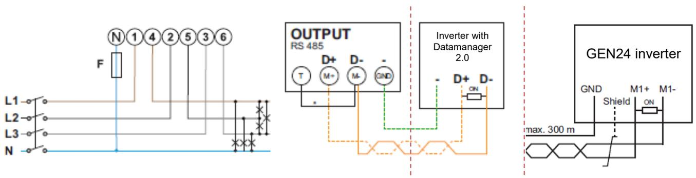
Contact T: 120 Ohm terminating resistor has to be bridged at the end of the Modbus line.
