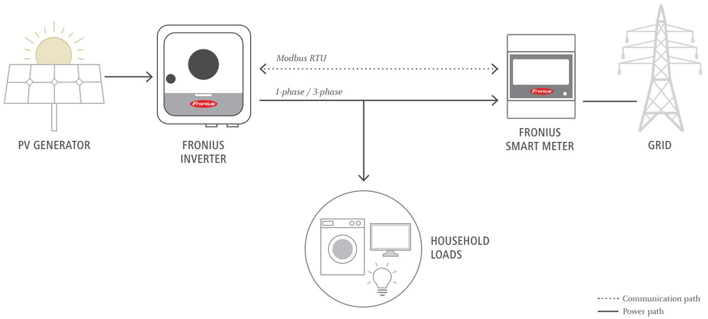
The Fronius Smart Meter is compatible with all inverters with an RS485 interface (Modbus RTU). The Fronius Smart Meter can be retrofitted at any time together with the Fronius Datamanager 2.0 in inverters that have already been installed.
