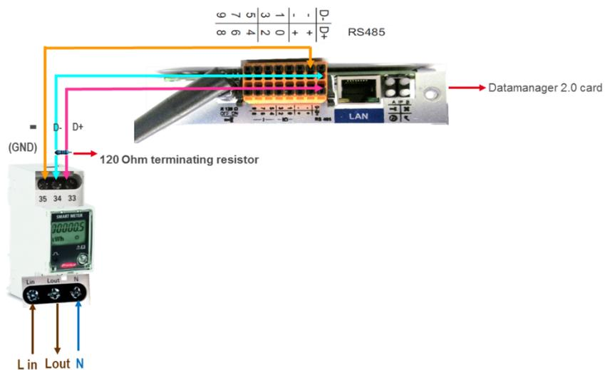
Figure 3: Wiring schematic - Fronius Smart Meter 63A-1
