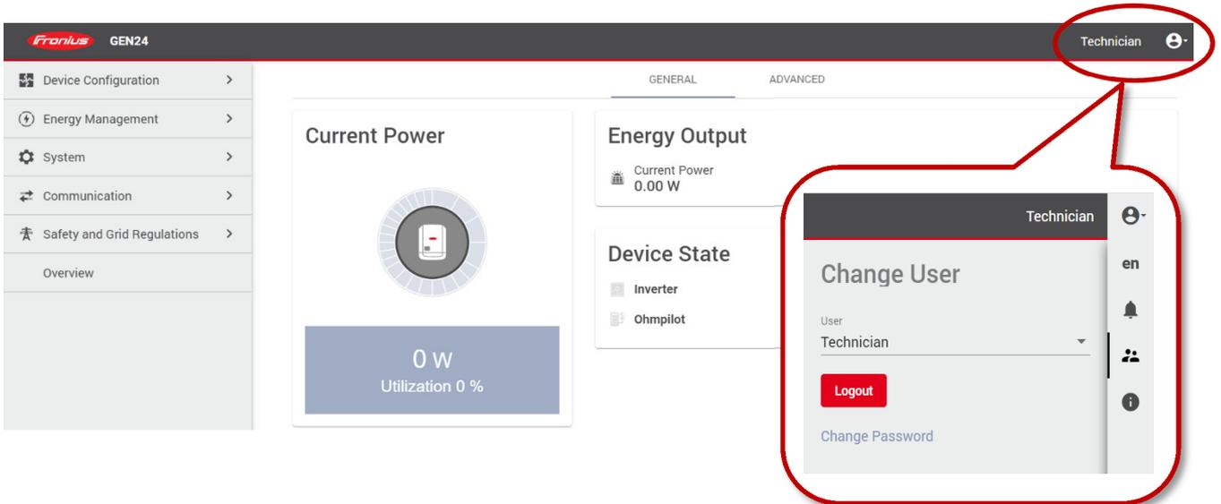
Enter the Submenu "Device Configuration" and go to "Components". There you are able to "add a component".
