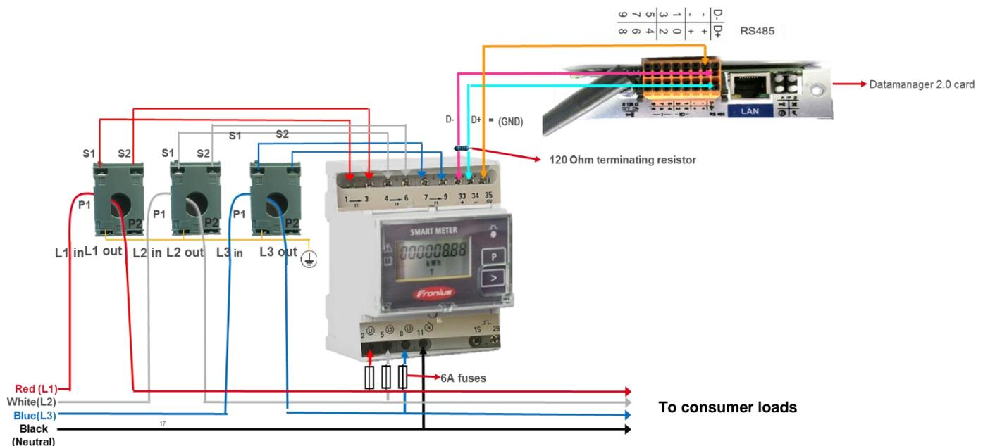
Figure 7: Wiring schematic - Fronius Smart Meter 50 kA - 3
