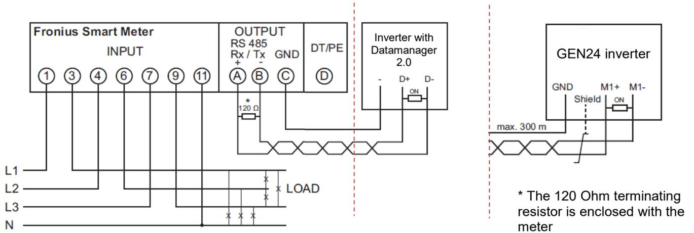
**Wiring detail for 3-Phase Fronius Smart Meter TS 65A-3**
