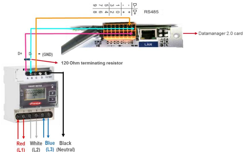
Figure 5: Wiring Schematic - Fronius Smart Meter 63A-3
