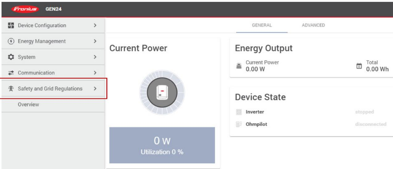
Enter "Export Limitation" and set the parameters "Total DC power of the entire system" and "maximum allowed feed-in power of the inverter" in % or Watt.
