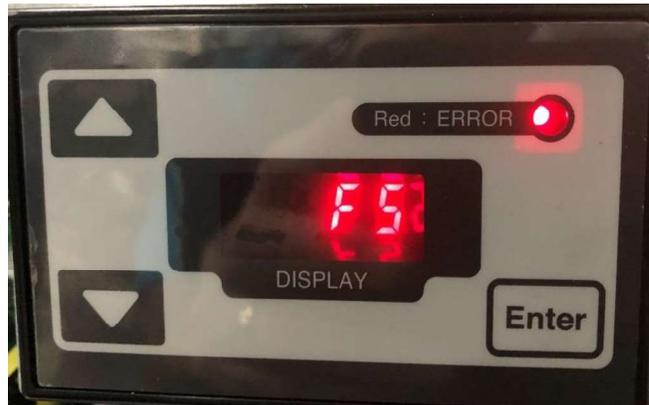
After a component is replaced or the inspection is completed, cycle power to the unit several times to confirm the error does not re-occur.
