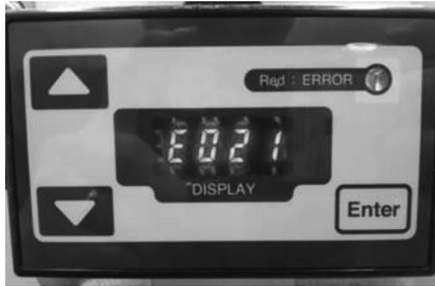
After a component is replaced or the inspection is completed, turn the breaker OFF for a period of 3 minutes before restarting to confirm the error does not re-occur.
