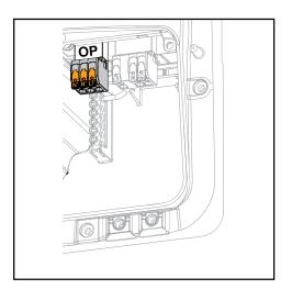
With the PV Point, in the event of a failure of the public grid, electrical devices can be connected to the Opportunity Power (OP) terminal and supplied with a maximum power of 3 kW, if enough power is available from the PV modules or an optional battery. In grid-connected operation, the OP terminal is not supplied with voltage, therefore the connected loads will not be supplied with power in this operating mode.
